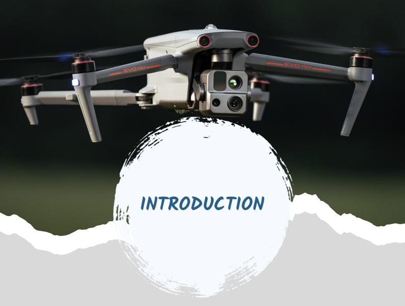
EVO Max 4T is the only commercial drone that combines traditional binocular vision systems with millimeter wave radar technology. This allows the EVO Max 4T's onboard Autel Autonomy Engine to perceive objects down to 0.5 inch, eliminating blind spots and enabling operation in low light or rainy conditions.
