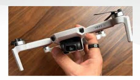
From a physical point of view, the DJI Mini 2 SE is almost identical to both the Mini SE and the Mini 2. It's a hair heavier than those two at 246g (including the battery, propellers, and a microSD card). The DJI Mini 2 SE is light enough to fly in the UK without a Flyer ID (you still need the Operator ID, though).
